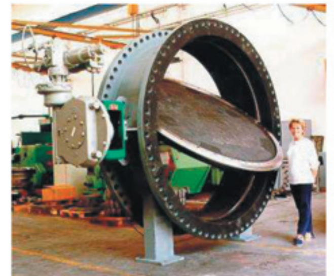
ND 3000 NP 6 fabricated carbon steel rubber lined body & disc sea water isolation MUARA TAWAR C.C.P.P. - INDONESIA
