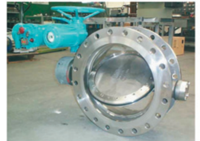
ND 24" ANSI 150, AISI 316L body & disc - sea water isolation JEBEL ALI DESALINATION PLANT - ABU DHABI
