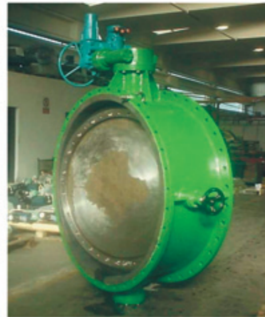
ND 1800 NP 10 carbon steel, rubber lined body, AISI 316L disc, with mechanical safety locking device CET 3 - PIOMBINO - ITALY
