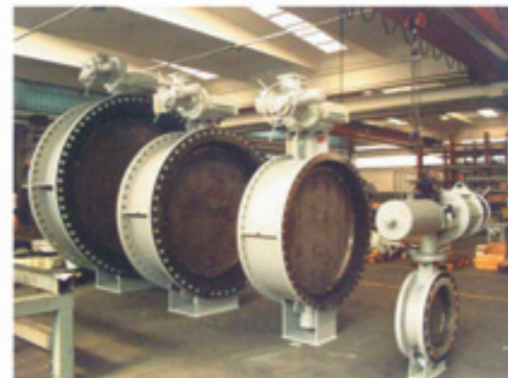
ND 24" ÷ 88" Cl.150 - carbon steel rubber lined body & cast titanium disc - sea water isolation UREA PLANT - AL JUBAIL - SAUDI ARABIA
