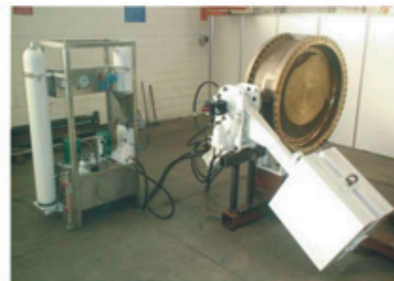
ND 48" ANSI 150 aluminium bronze body & disc sea water pump protection and isolation VINIL QATAR PROJECT
